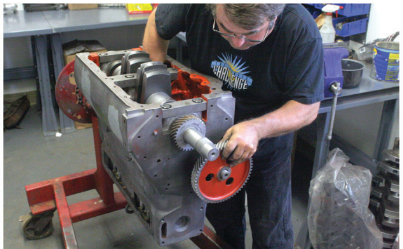
Baker carefully feeds the camshaft into the engine and aligns the cam and crank gears in proper sequence.
