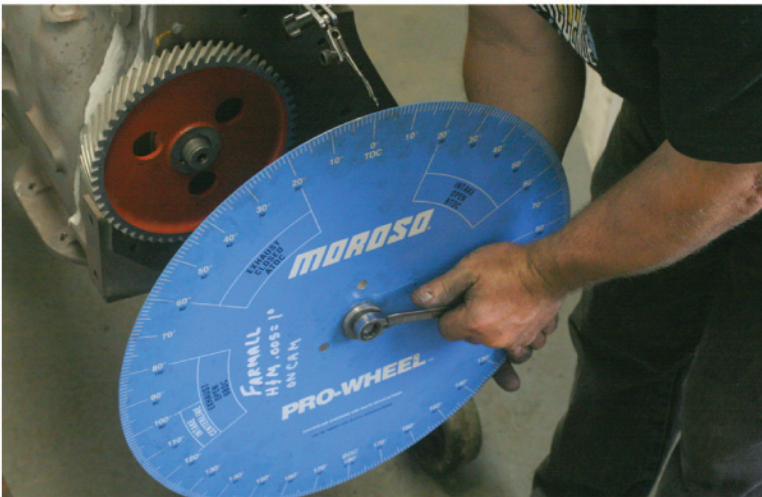
Having gotten the piston close to TDC, Gary tightens the degree wheel and aligns the pointer to zero "0."
